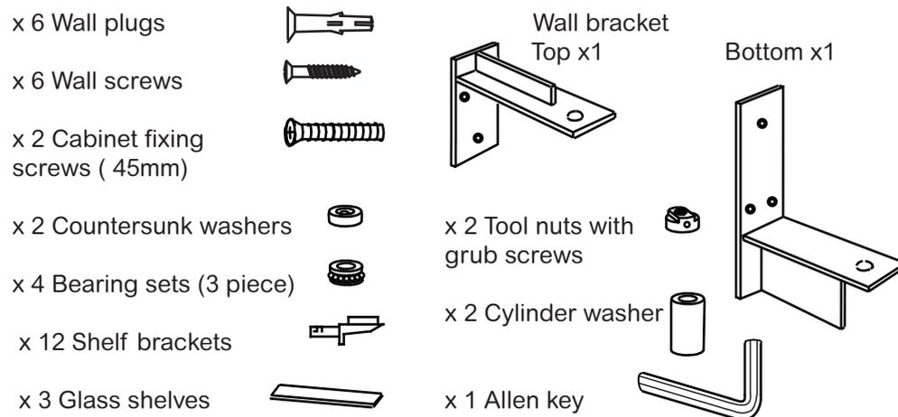
You will need a power drill, masonry drill bit, cross-head screwdriver, spanner, tape measure, spirit level and pencil to install this product. Ensure the wall surface is of suitable strength and construction before fixing the cabinet.
