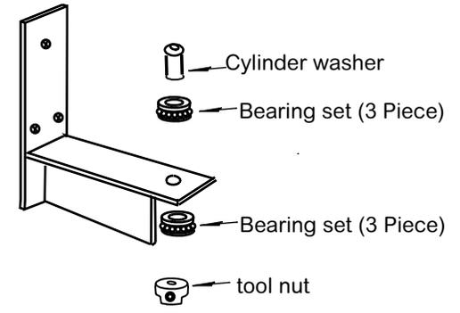
4 Tighten tool nut and grub screws securely
